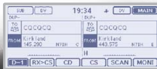
DV/DV dualwatch (DR function) example
