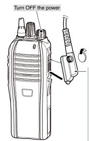
CAUTION: Attach the multi connector snugly, but do not overtighten. A loose connection will allow water intrusion into the connector. A overtightened connector will damage the connector pins in the transceiver.
