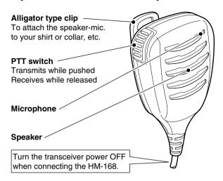
**NEVER** immerse the connector in water. If the connector becomes wet, be sure to dry it BEFORE attaching it to the transceiver.
