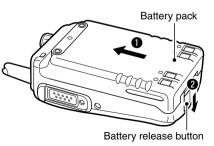
**NOTE:** Keep the battery pack terminals clean. It's a good idea to clean the battery pack terminals once a week.
