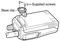
② Clip the belt clip to a part of your belt and insert the base clip into the belt clip.
